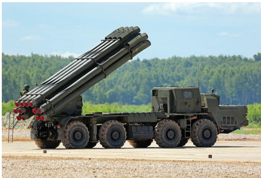
Figure 12: The BM-30 Smerch, a Russian heavy multiple rocket launcher. Source: Shutterstock/ID1974.
